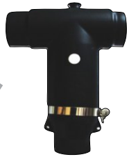
36 kV BIL 200 Elbow connector 630A (Front) Interface C EN 50180. XYZ=Cable Data ordering information
