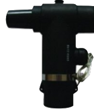
36 kV BIL 170 Elbow connector 630A (Rear) Interface C EN 50180. XYZ=Cable Data ordering information
